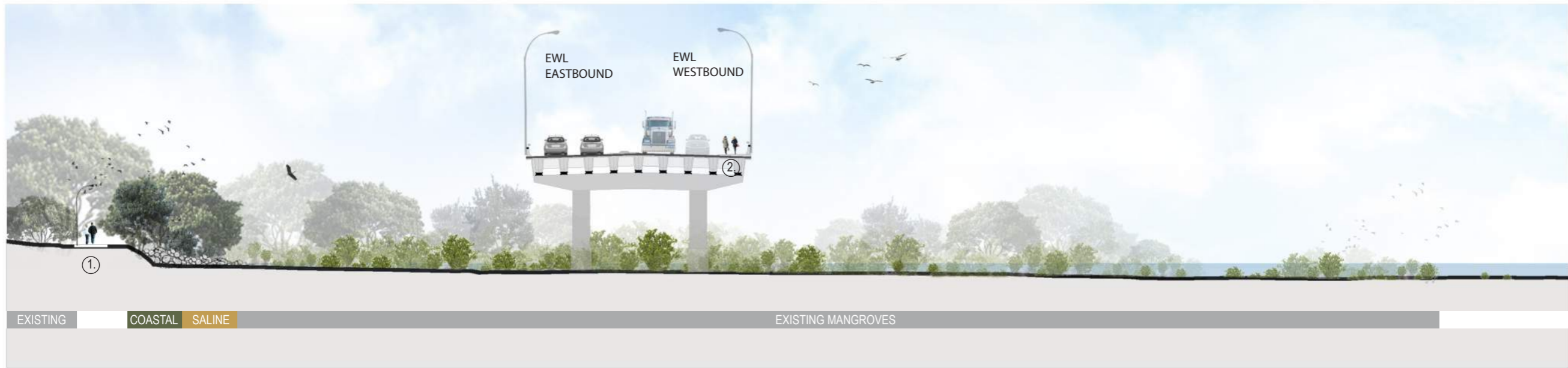
ANNS CREEK - 2D SECTION (A7) CH4050 SCALE 1:500
