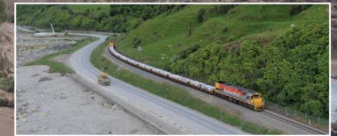
As the rail line became functional again, it was used to assist the road rebuild moving supplies and equipment – including five-tonne seawall blocks to site. KiwiRail has only been running trains at night so road and rail works can be done quicker.
