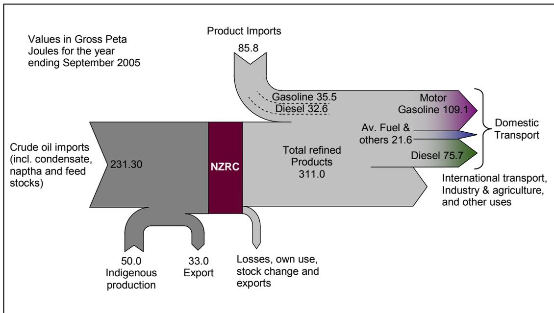
Figure 3.7 Typical transportation fuel supply and distribution for New Zealand 2005<sup>9</sup>.
