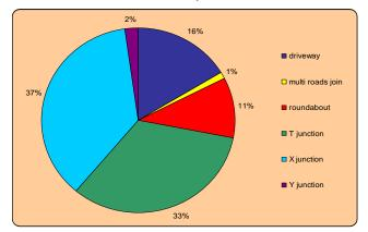
Sixty percent of intersection and driveway crashes between 1999 and 2003 involved a collision between vehicles making either a crossing or turning movement. Eighty-nine percent of these involved a vehicle failing to give way or stop.
