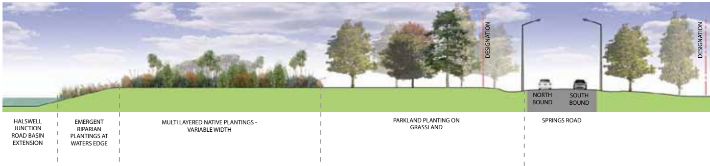
SPRINGS ROAD/HALSWELL JUNCTION ROAD BASIN EXTENSION Figure 43: Cross-section J-J (CH 100). Scale 1:400
