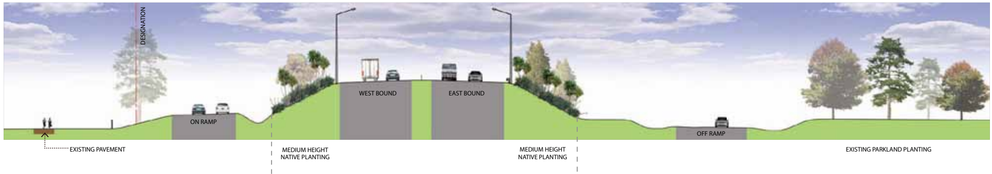
CURLETT'S ROAD INTERCHANGE Figure 60: Cross-section D-D (CH 7250). Scale 1:400
