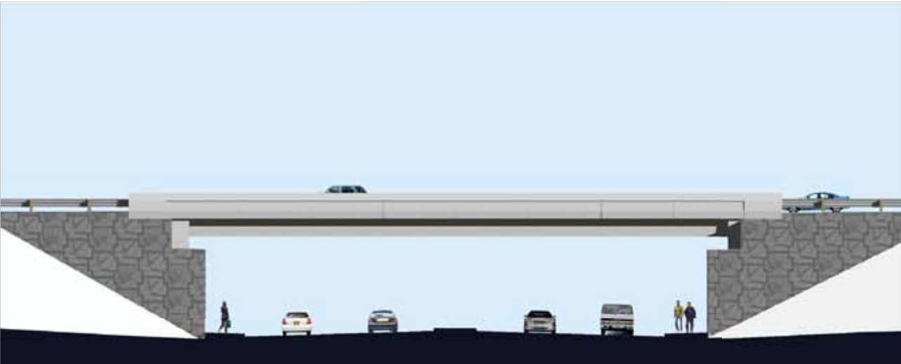
Figure 96: Elevation of bridge showing MSE wall
