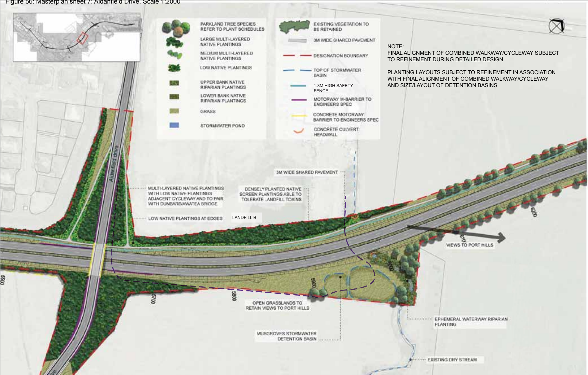
Figure 56: Masterplan sheet 7: Aidanfield Drive. Scale 1:2000
