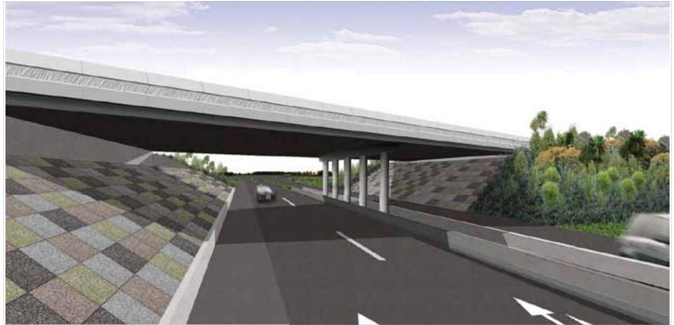
Figure 98: Perspective view of Curletts Road Overpass showing potential spill through surface treatment
