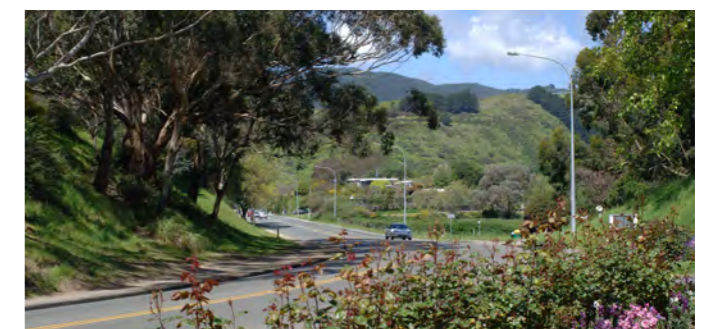
Figures 36 and 37 Poplar Avenue above and Raumati Road - photos show how these roads were developed as cuts through dunes - the roads extend from the existing SH1 in straight lines to these inland dune points
