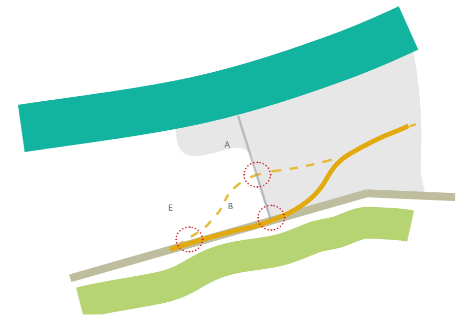
At the south end the preferred option requires only one over bridge at the end of Poplar Ave (B) - the alternative would have required two bridges - 1 in the park (E) and the other on Poplar Ave in the proximity of residential and school uses. The preferred options also locates the bridge at the beginning of the Raumatī urban area (A) - this is considered a more legible place to signal the arrival point and where a choice can be made to divert to the Paraparaumu town centre along the former SH1
