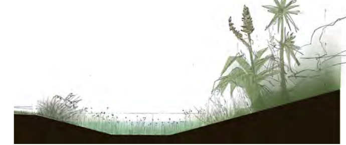
Figure 107 Storm water swales
