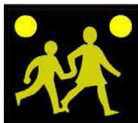
Figure. Example of a school bus sign incorporating two alternatively flashing lights.
