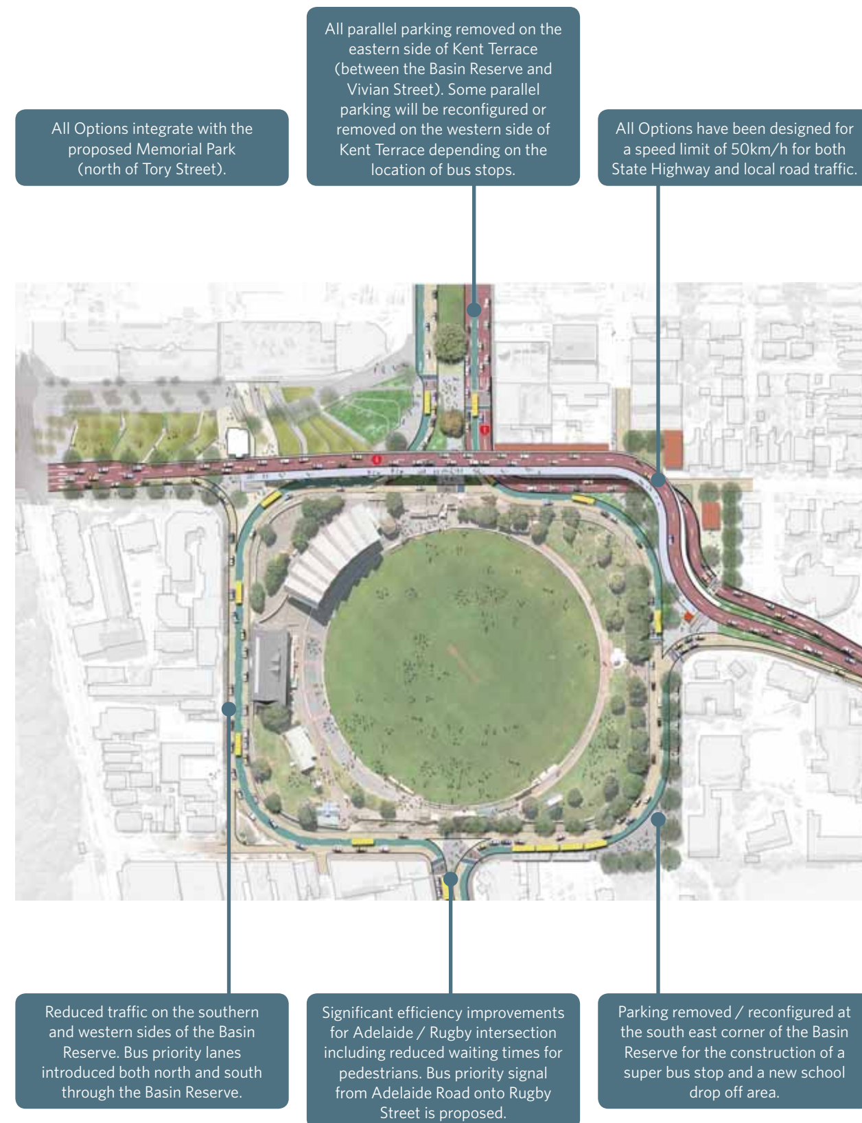
Figure 2.6: Shared Characteristics of each Option (Option A used as an example)
