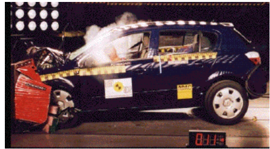
Offset crash test at 64km/h
