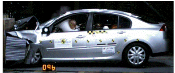
Offset crash test at 64km/h
