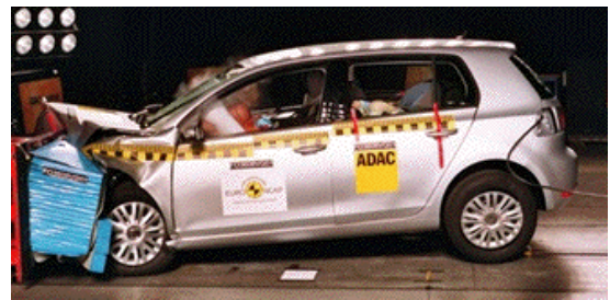
Offset crash test at 64km/h
