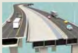
3 NEW 3 LANES SOUTHBOUND IN USE EXISTING SOUTHBOUND LANES VACATED CONSTRUCTION FOR 4TH LANE TIE-INS AT NORTH AND SOUTH APPROACHES
