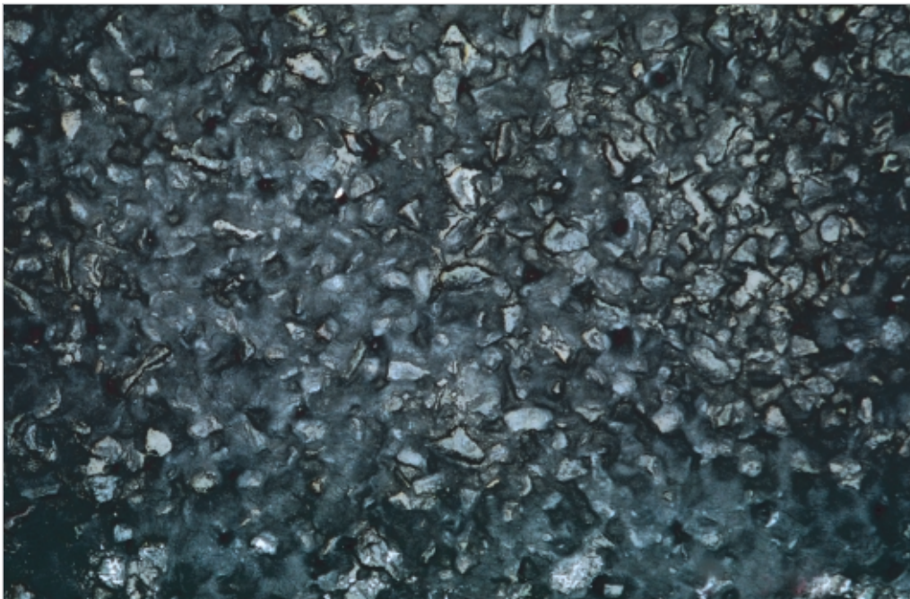
Figure 12-1 Small holes are evidence of binder rise through the action of vapour venting (volcanoes) (see also Figure 4-20).
