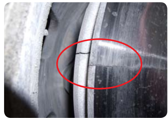
Cracking through rotor surface area - unacceptable
