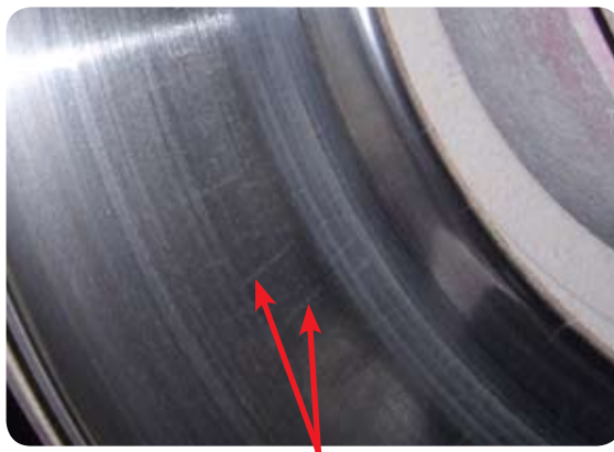
Minor heat cracking - acceptable
