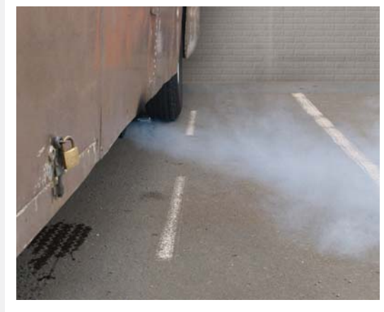
Figure 5. Clearly visible smoke. This vehicle would fail.
