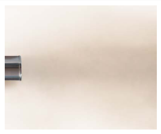
Figure 2. Clearly visible smoke. This vehicle would fail.
