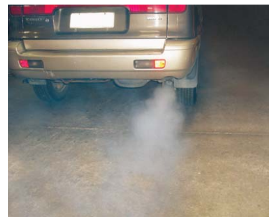
Figure 4. Clearly visible smoke. This vehicle would fail.
