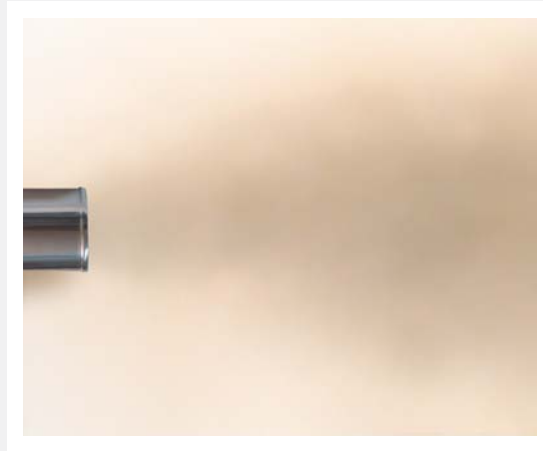
Figure 3. Clearly visible smoke. This vehicle would fail.
