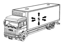
Thus the stability of a truck is largely dependent on the height of its CG above the ground. If a load is not centred across its width; the stability will be reduced when cornering.
