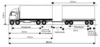
Begin by considering the load space requirements when working out the configuration. Engine size doesn't matter, that comes later.
