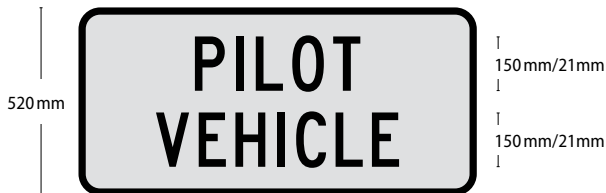
Figure 17. Warning sign for pilot vehicle
