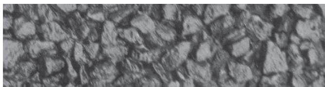
Coating D, total bitumen film thickness 110 microns
