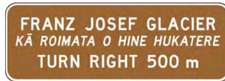
FIGURE 1.13: A TYPICAL DUAL NAME TS-2 TYPE (Secondary name is longer than the primary name)
