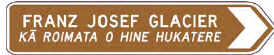
FIGURE 1.14: A TYPICAL DUAL NAME TS-2 TYPE ADVANCE SIGN (Secondary name is longer than the primary name)
