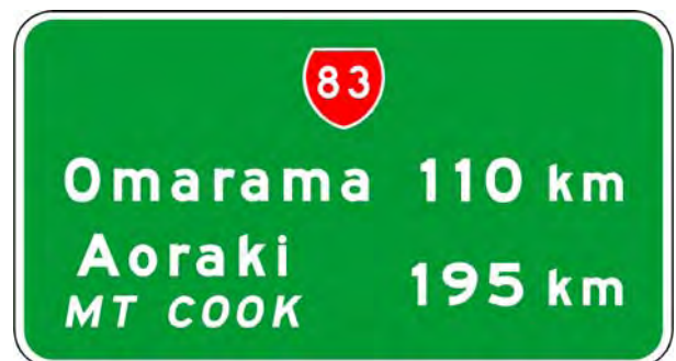
FIGURE 1.9: A TYPICAL DUAL NAME CD-1 TYPE CONFIRMATION DIRECTION SIGN (Secondary name longer than primary name)
