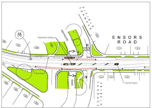
Figure 4.37 Ensors Rd pedestrian facility layout plan
