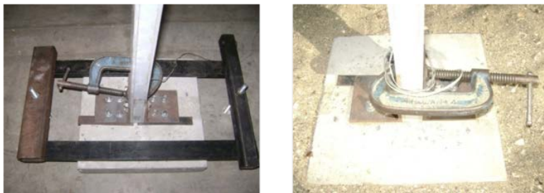
Figure 5.2 Foundation conditions: (a) Fixed base and (b) field test foundation (concrete footing on sand)
