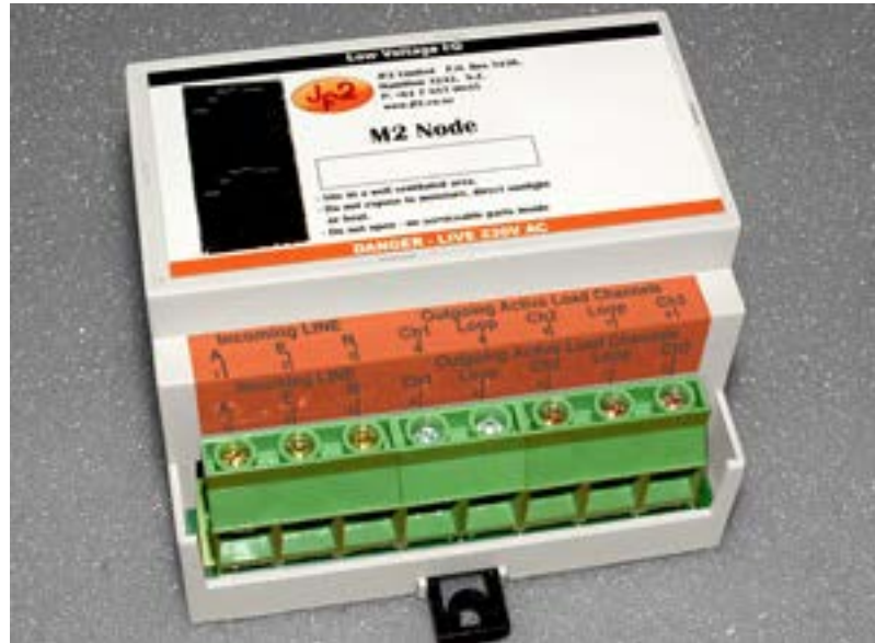
Figure 43 LATA Lighting Control Module (Source: Website)
