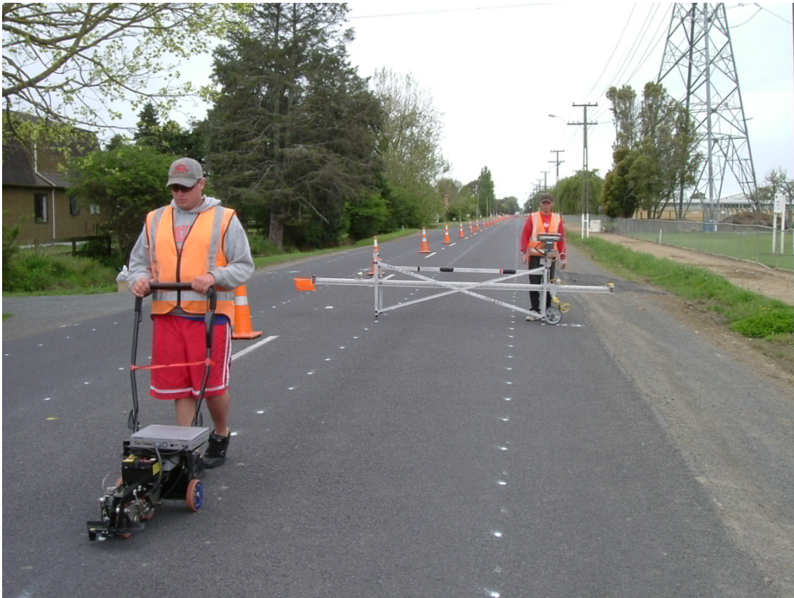
Figure 1: Transverse Profile Beam and Walking Profiler.
