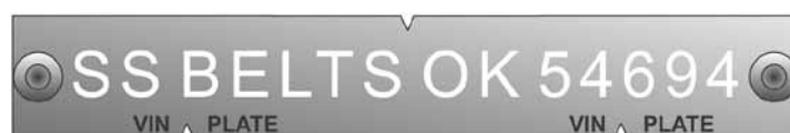
Figure 1. Example of a plate fitted to a vehicle that may retain a single-sensitive seatbelt
