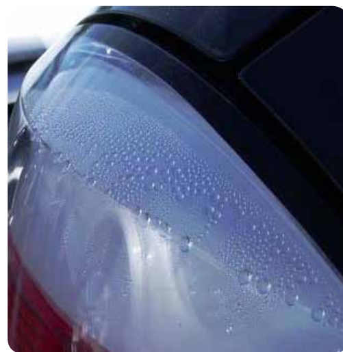
Figure 2: Heavy moisture - large droplets - FAIL
