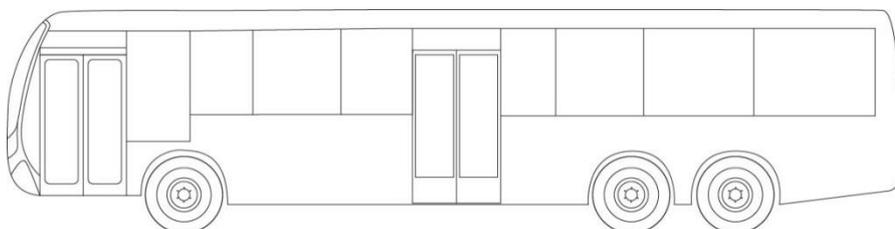
This form of vehicle is in wide use for urban bus services. A typical vehicle has three axles, with a total length of 13.5 m. These vehicles are already allowed a slightly longer overhang (the distance between the last axle and the back of the vehicle) than other heavy vehicles. Effectively, these vehicles are at the limit of length versus their ability to fit on the available road network, especially in suburban areas.
