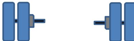
Some heavy vehicles replace two standard tyres with a single wider tyre (a “single large” or “mega” tyre).
