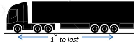
The engineering principle is that if a given gross mass is distributed over greater length, it reduces the effect on bridge spans.
