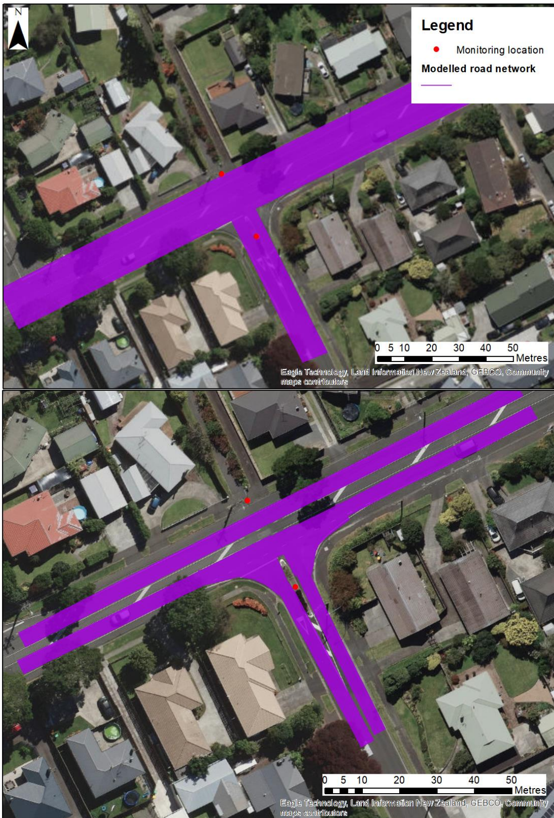
Figure 5-2: Example of modelled road network refinements around a junction to better represent the widths and alignments of the road network.
