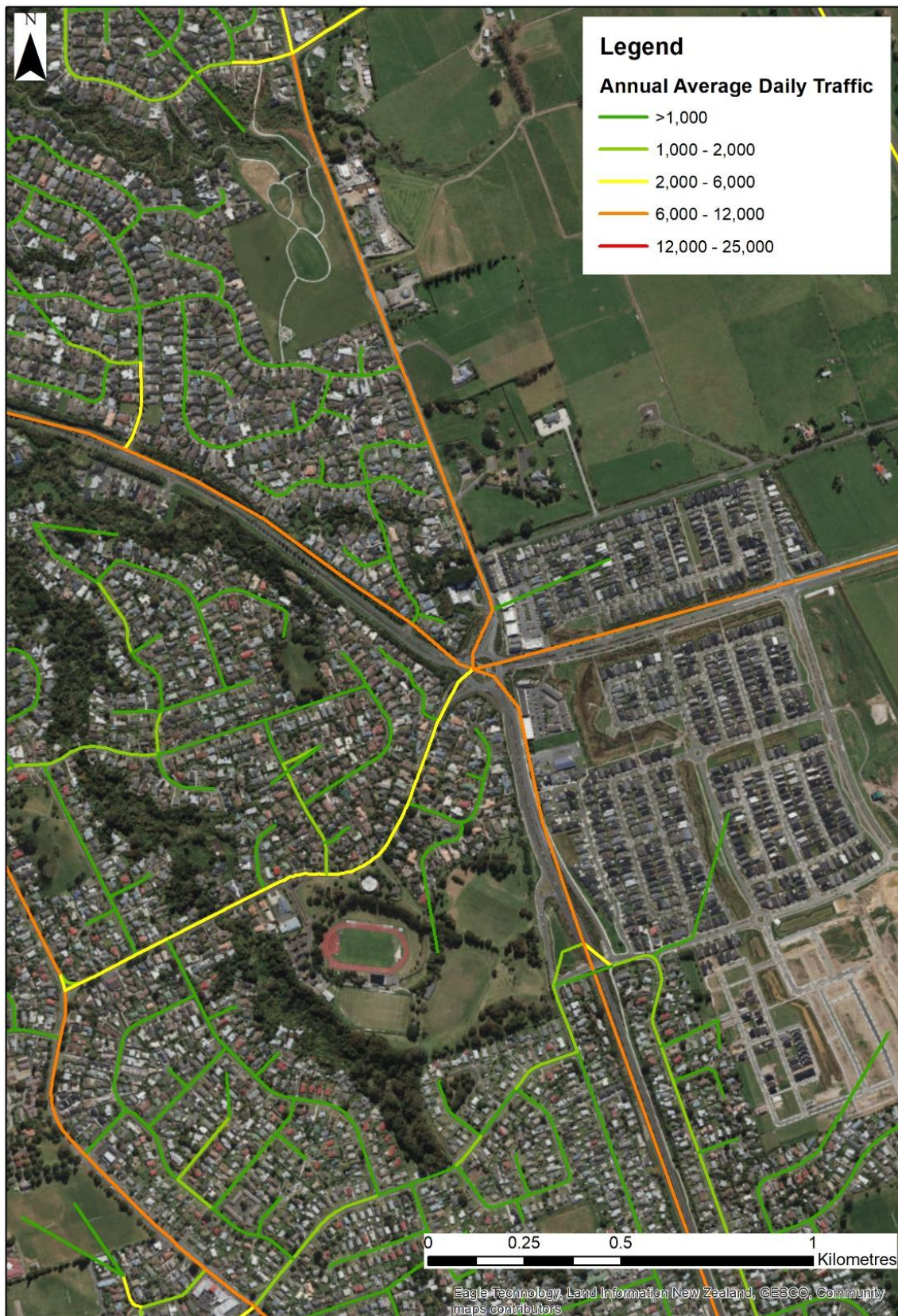
Figure 5-3: Example of the use of colour banding symbology to investigate traffic flow volumes.
