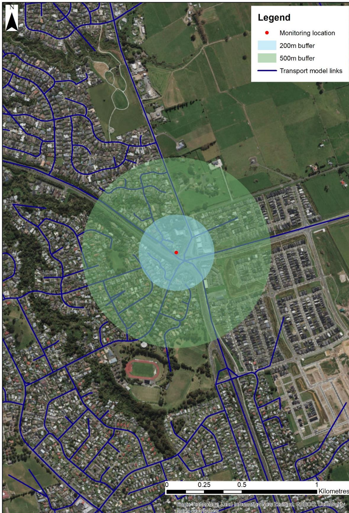
Figure 5-1: Example of the use of buffers to ensure 500m extent around a monitoring location.
