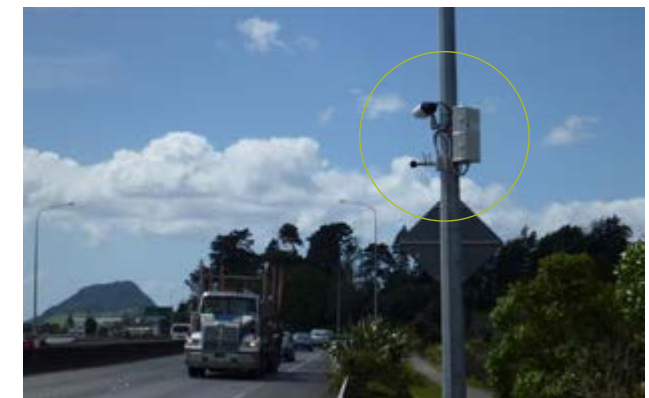
The Transport Agency has trialled a 'noise camera' in Tauranga (2013/2014). The system has a microphone to trigger a camera which reads the number plates of trucks with particularly noisy engine brakes.
