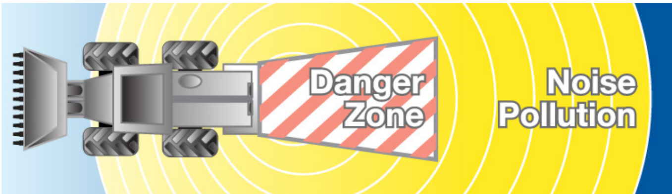
Broadband alarms generate warning noise in the danger zone but less spilled noise than tonal alarms
