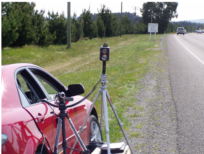
Figure 3: The radar gun and video camera in use at site 5
