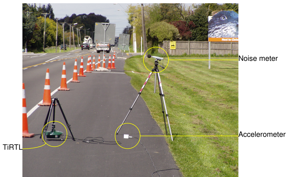
Figure 1: The TiRTL (lower tripod), noise meter (tall tripod) and accelerometer (little white box on road) installed at site 4, Christchurch - bound side of the road.
