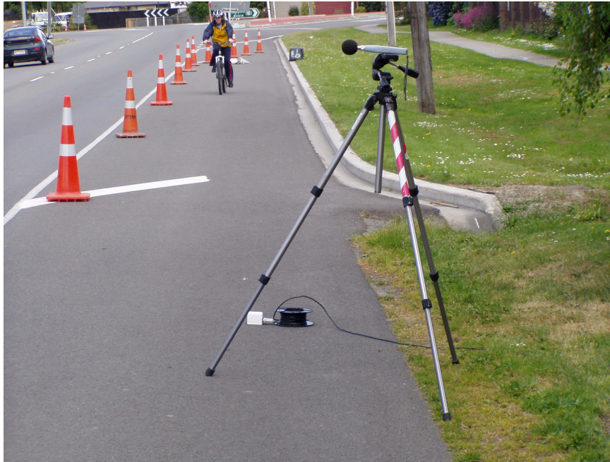
Figure 2: Noise meter (tall tripod) and accelerometer (little white box on ground) as installed at site 3, landfill – bound side of the road
