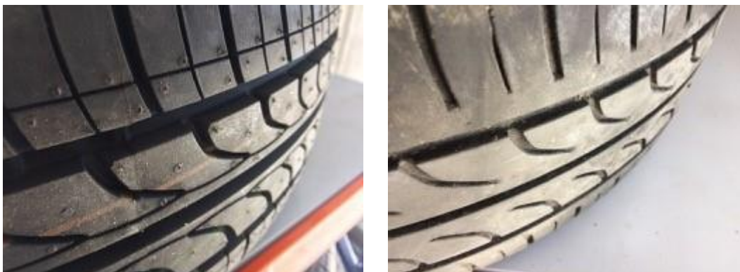
Figure 2-1: The 'typical' tyre, Bridgestone Supercat 195/60R15, in new (left) and worn (right) condition
