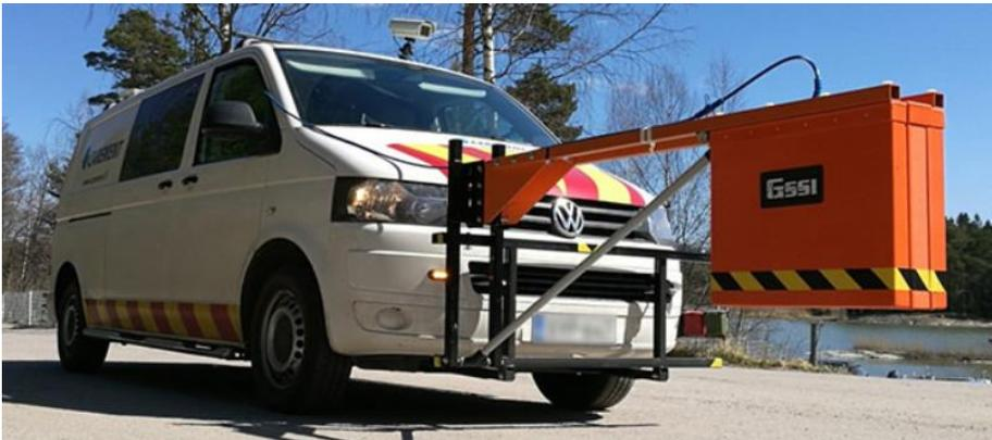
Figure 4. Vehicle mounted GPR system.
