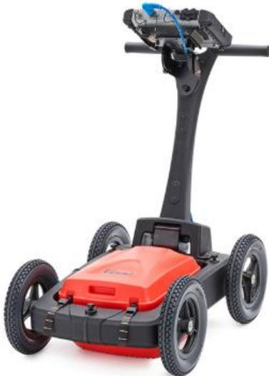
Figure 5. Push-along GPR system.
