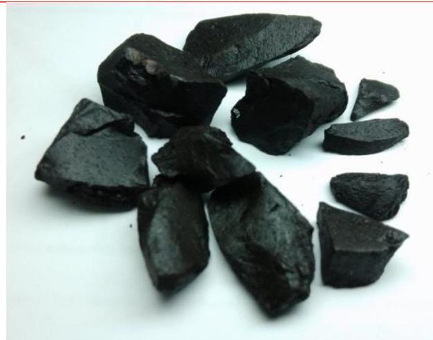
Figure 2: Trinidad Lake Asphalt (source: Nicri et al. 2014)
