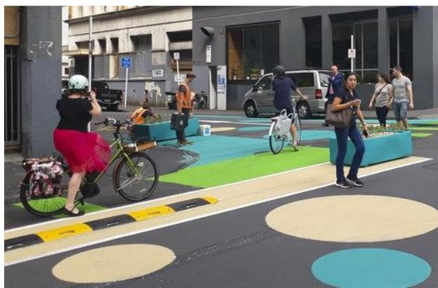
**Figure 13: rubber speed humps, paint and plastic planter boxes delineate space, Auckland**
