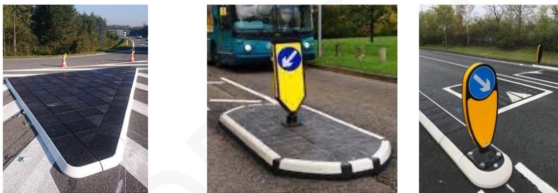
**Figure 21: traffic islands made of interlocking rubber elements (left, centre) and separator kerbed islands with speed cushions (right)**
