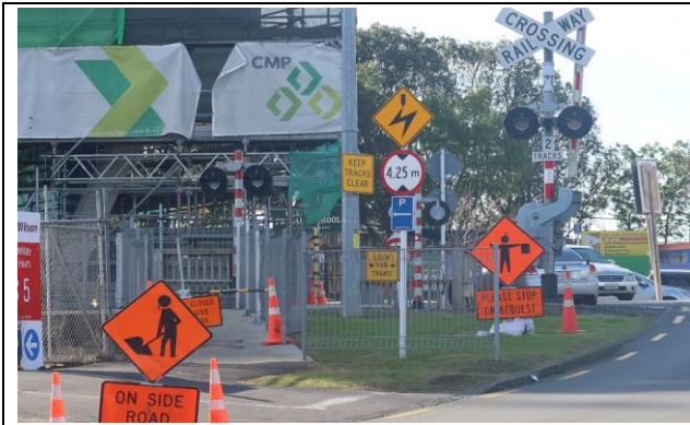
Example of confusing signage as approaching a level crossing.
