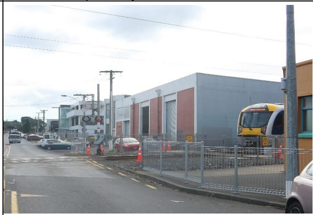
View of signalling when crossing is activated on the wrong side of the road (half-arm barrier has very low visibility and flashing lights are not observable)
