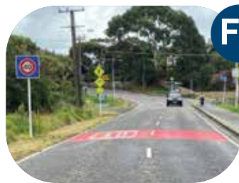
Flush Threshold treatment, e.g., 30/50
