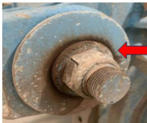
**Figure 2:** These black marks shouldn't be present on a secure connection. If they are, replace the pin kit and bushes.
