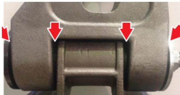
**Figure 1:** A rubber bead should be formed in each area the arrows are pointing to, separating the metal components. It should be complete around the circumference and not split.
