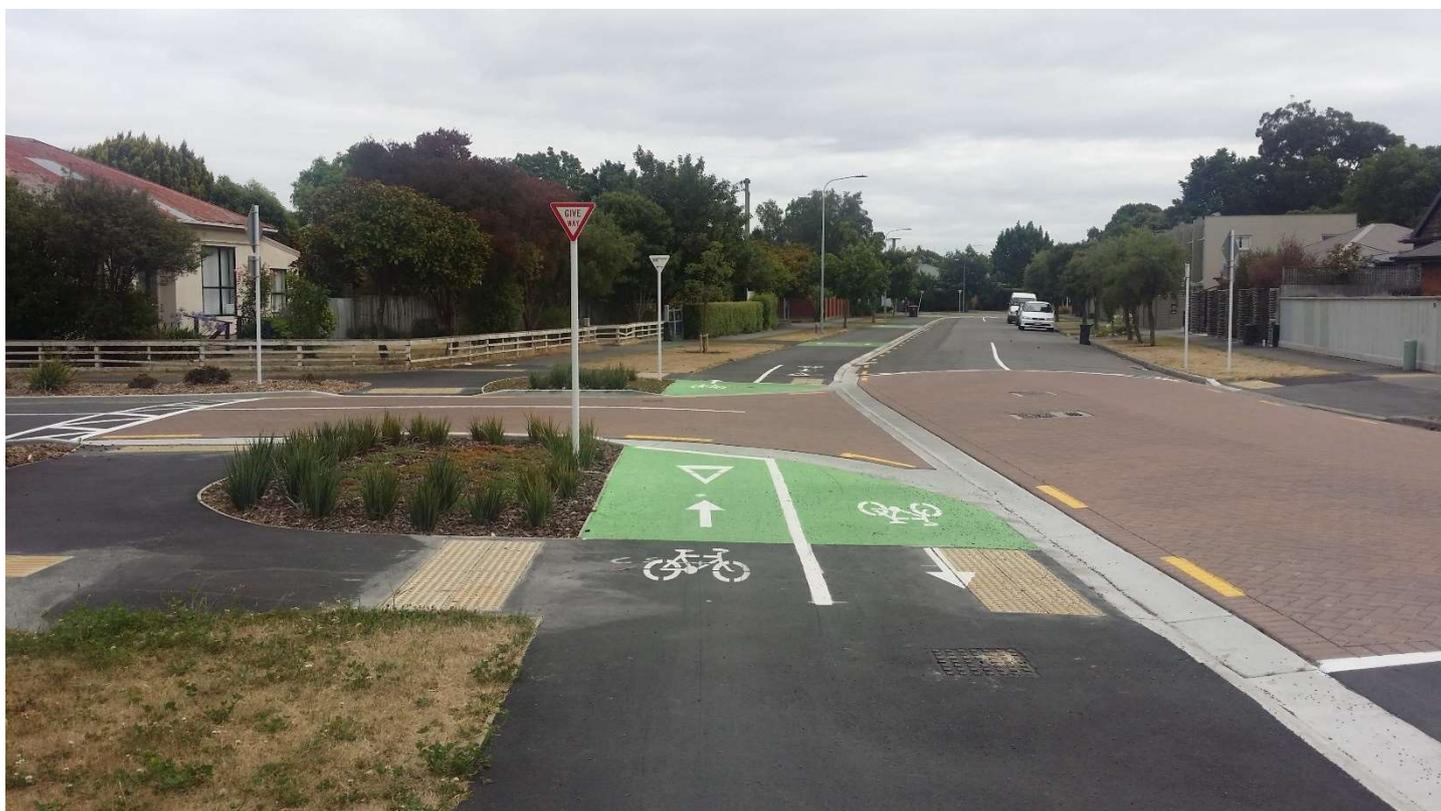
Figure 12: Straight through cycleway where cycleway users are to give-way to motor traffic
