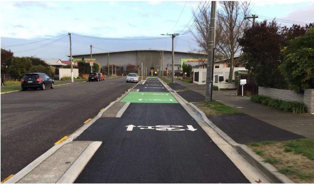
**Figure 14: Separated bi-directional cycleway without adjacent parking at a residential driveway**
