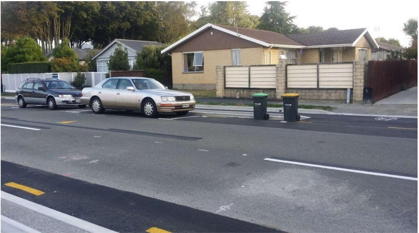
**Figure 17: Applying setbacks for parking at driveways along separated cycleways, Strickland St, Christchurch**
