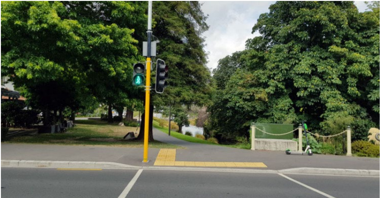
Figure 29: Pedestrian-only signal display. (Photo: Gemma Dioni)
