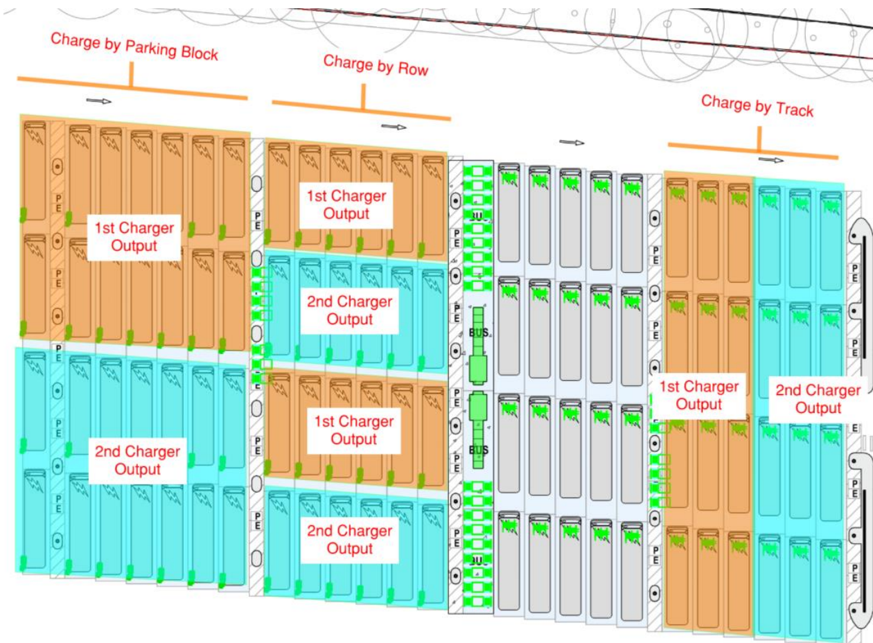
Figure 20: Conceptual bus depot layout showing different charging strategies (Source: Transport Canberra)
