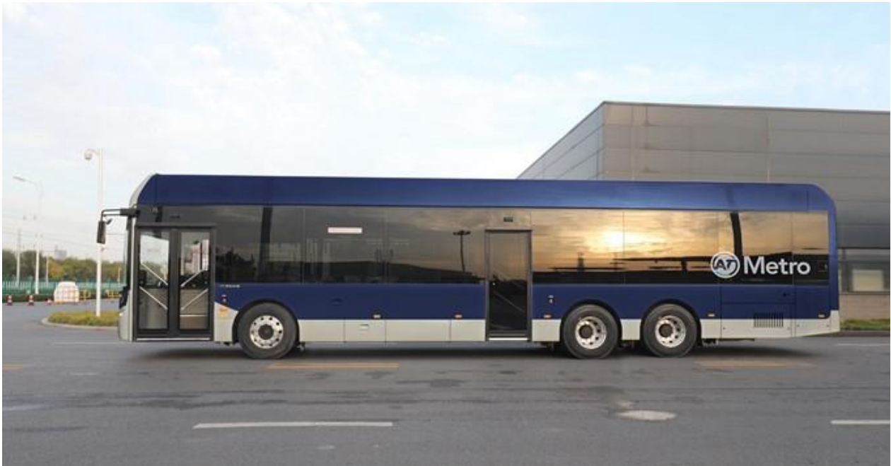
Figure 3: Three axle battery electric bus used in Auckland (Source: Auckland Transport)
