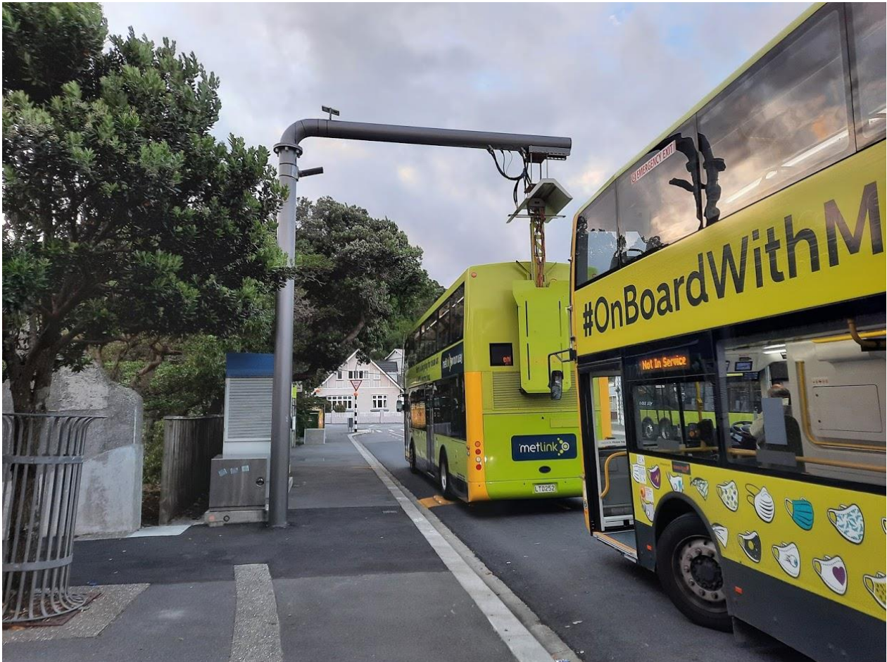
Figure 39: Battery electric double deck bus with pantograph opportunity charger (Source: Lorelei Schmitt)
