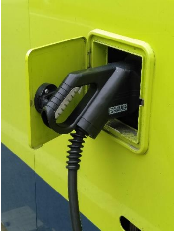
Figure 19: A bus charging using a plug connection (Credit: Kirsten Boardman)
