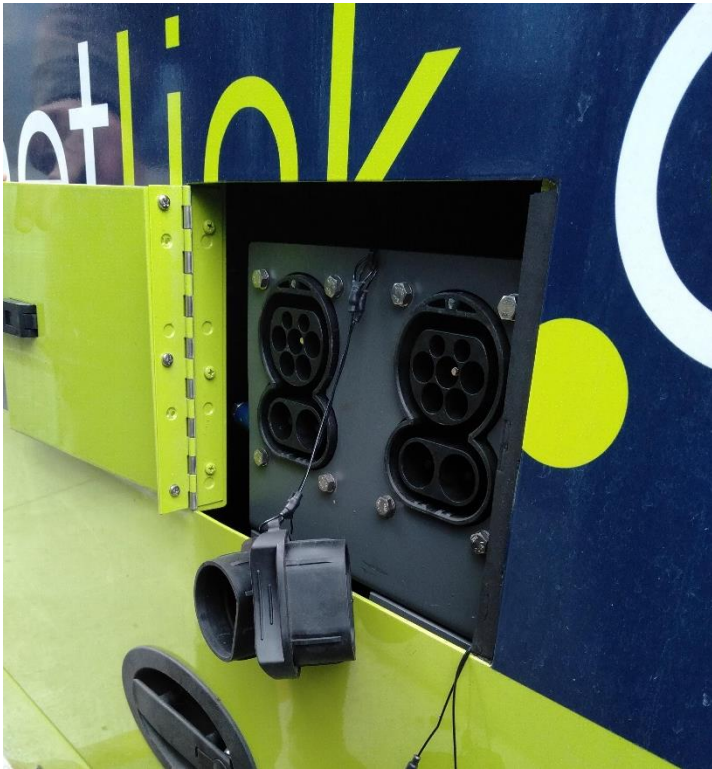
Figure 5: A bus with multiple charging ports (Credit: Kirsten Boardman)
