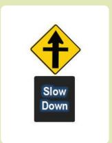
Sign 1 combines an existing intersection warning sign (PW-9) with an active LED sign that displays the words 'Slow Down', which would flash at an appropriate frequency (for example, 1-second cycle time)
