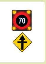
Sign 2 combines an LED active sign unit as used for 40km/h school signs (including flashing amber beacons) modified to display 70km/h with an existing intersection warning sign (PW-9).
