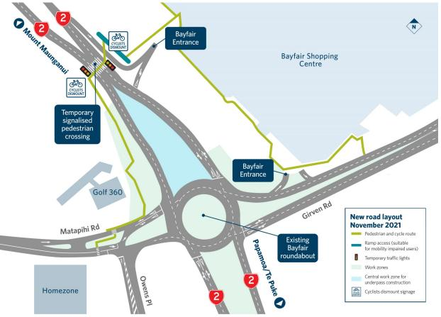
The new central work zone will enable construction to proceed on the underpass' middle section (an open-air trench), two further piers for the four-span Bayfair flyover and the flyover's northern embankment.
