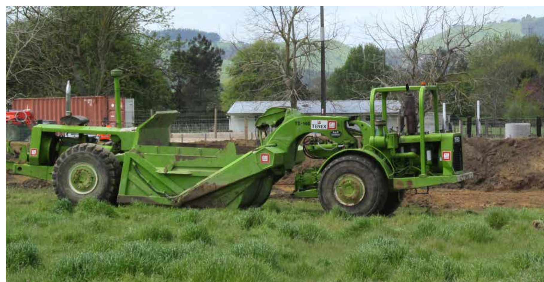
This scraper scoops the ground beneath it to pick up dirt and move it somewhere else
