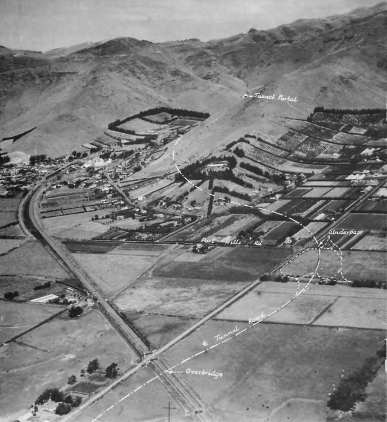
*Showing route to the portal of the Christchurch side of the road tunnel. The railway leading to the present tunnel leads through the middle of the photograph.*
