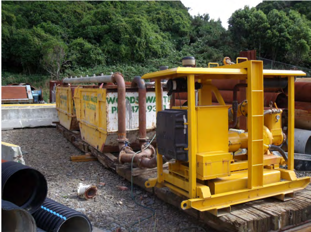
Plate Ten – Mobile Polymer Mixing and Pumping Unit
