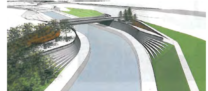
Figure 89 Concept of wrapping the under bridge abutments out into the landscape beyond
