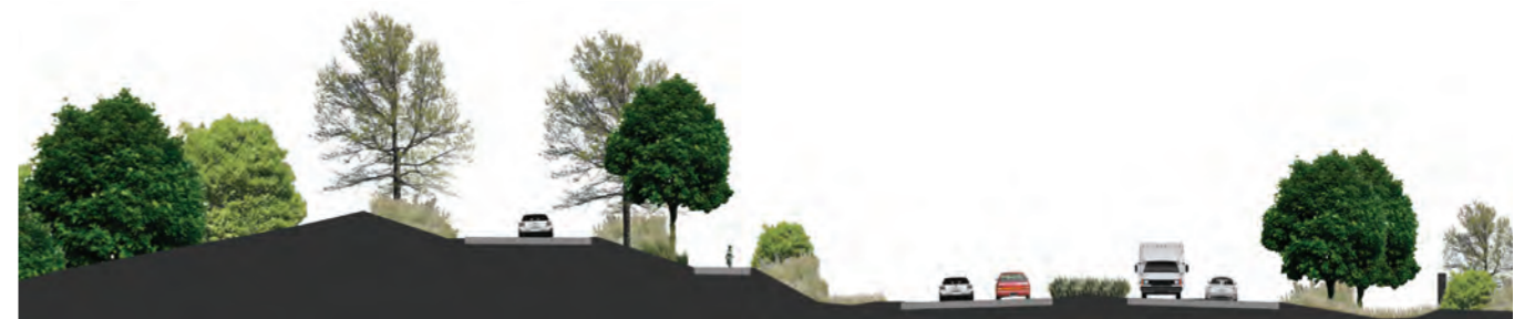
Figure 98 (Above) Cross-section describes the building up of the ground to use the rise as part of the noise reduction block. This section is north of Leinster Ave with the Expressway on the right and residential property to the far left. The cycle path and service lane are part way up the slope.
