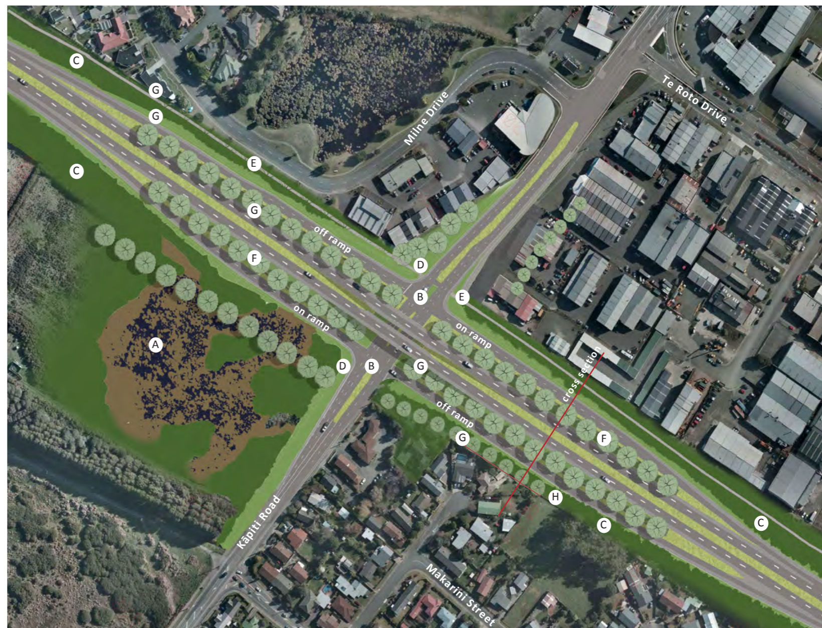
Figure 135 At Kāpiti Road showing proposed landscape integration by utilising clear stemmed native specimen trees in conjunction with dense planting under. Walls can also be greened with climbers
