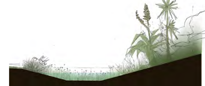
Figure 107 Storm water swales
